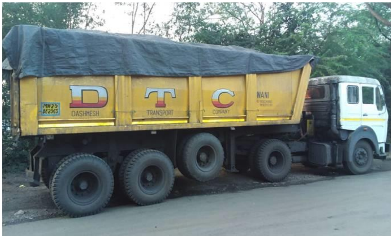
Coal transportation by truck wagon with tarpaulin covering
